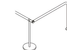
The end caps for border rails are always necessary when attaching corner joints or intrusion prevention bars to bases.
