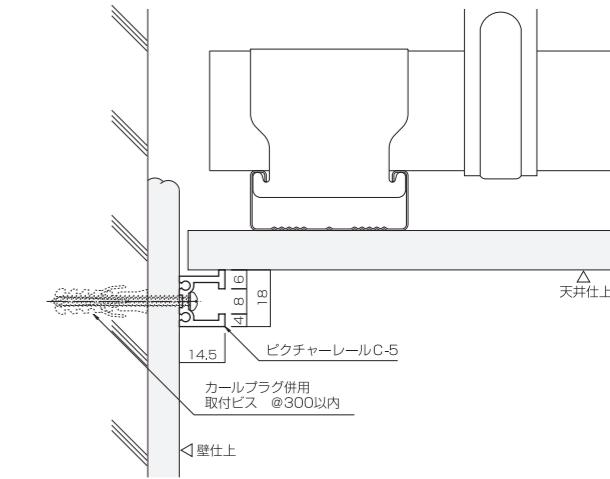
**C - 2D** GL工法壁 取付例 GL method of construction wall
