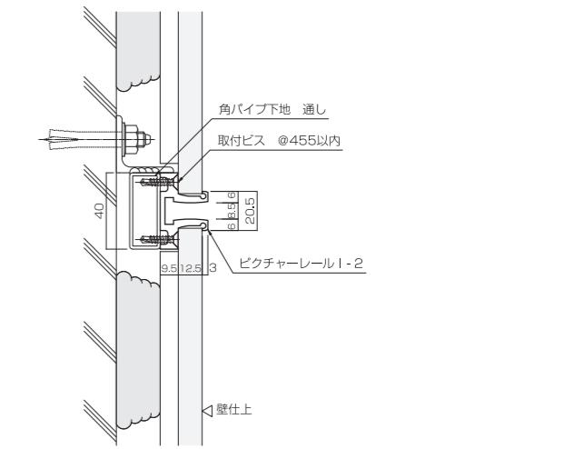
I - 1 GL工法壁 取付例 GL method of construction wall
