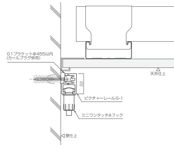
G - 1 軽量鉄骨壁 取付例 Lightweight steel frame wall
