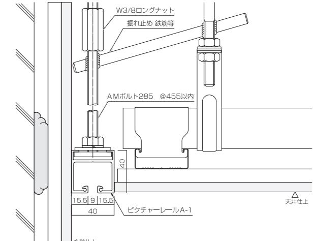
A - 1A GL工法壁 取付例 GL method of construction wall
