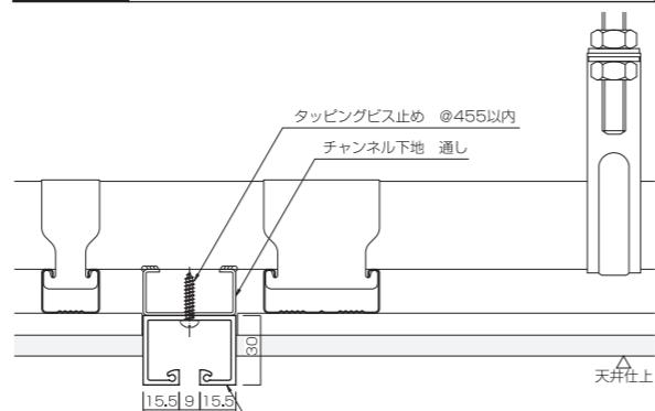
D - 1A 軽量鉄骨壁 取付例 Lightweight steel frame wall
