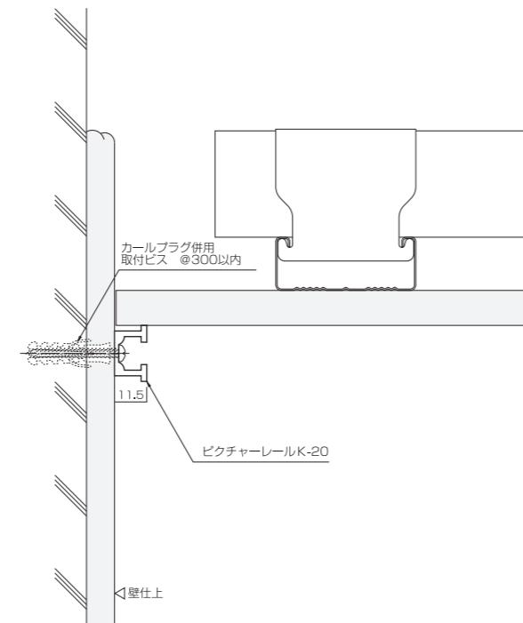
K-20A 軽量鉄骨壁 取付例 Lightweight steel frame wall
