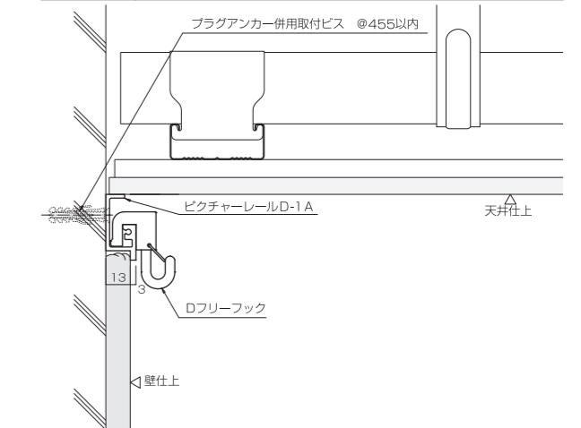
D - 1B GL工法壁 取付例 GL method of construction wall
