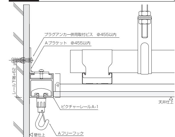
A - 1 GL工法壁 取付例 GL method of construction wall
