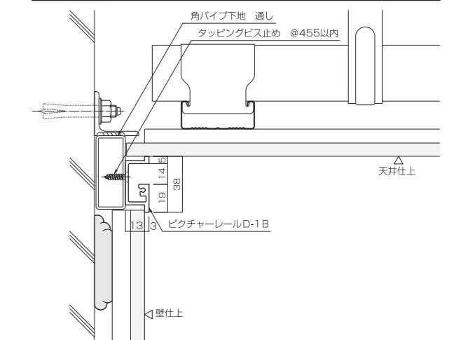
D - 1B 軽量鉄骨壁 取付例 Lightweight steel frame wall
