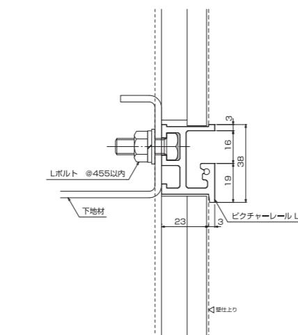
L - 1 軽量鉄骨壁上部取付例 Light weight steel frame wall
